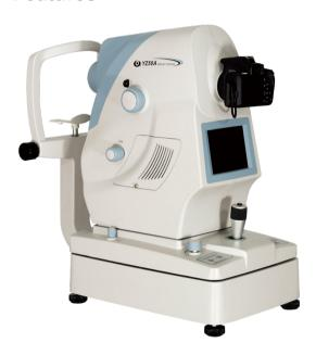
The YZ50A Serious Non-mydriatic Fundus Camera is used to observe and photograph the posterior segment on the eye including retina,macula and posterior pole. The instrument uses infrared light as the illumination source, has focus split indicator showing the amount of focus deviation in the fundus observation screen, also locates the accurate position by using pupil positioning spots. The instrument is easy to operate, flexible and reliable for medical use.
